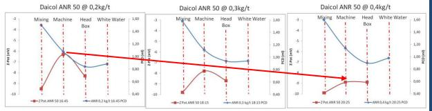
From the analysis of Z-potential and PCD values during trial, we can see a first effect of Daicol ANR 50 as "fixing agent" of cationic starch. Further additions of Daicol ANR 50 show a good fixation of the product (minor impact on PCD values, higher impact on Z-Potential) that help to keep the strength of the paper, despite a quite high increase of the ash content in the paper.
