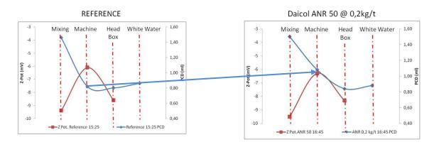
The main effect of a small addition of Daicol ANR 50 is on PCD of Machine chest. Cationic demand increase from 0.82 mL to 1.08mL while in the other sampling points PCD remain almost the same. Daicol ANR 50 adsorbed on fibers result in a better fixation of cationic starch as seen during laboratory evaluation.
