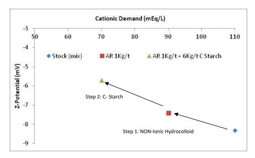
Delta of Z-potential after addition of 6 kg/t of Cationic Starch (step 2) is **+ 2.7 mV** using our anionic hydrocolloid, while delta of Z-potential is **+ 1.7 mV** after addition of NON -lonic hydrocolloid.
